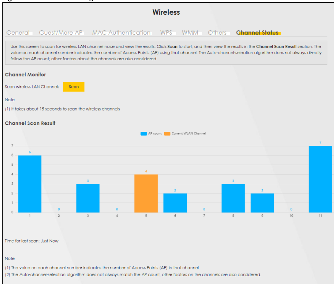
Figure 63 Network Setting > Wireless > Channel Status
